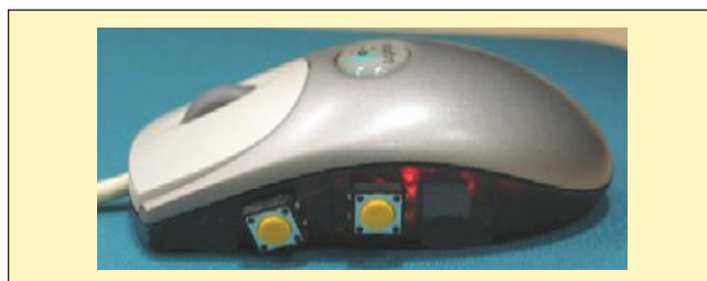
Figure 5. Vibrotactile mouse used to display the haptic icons used in the turn-taking protocol. Two buttons were added to the side to enable special protocol features; such buttons were available in other mice at the time but not the vibrotactile one.
