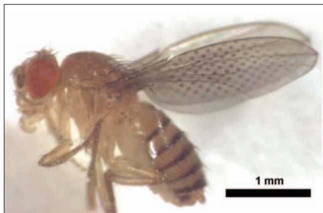
Figure 18. Live Drosophila after thermal evaporation carrying a pattern of 100-nm-thick, 50- \mu\text{m} -wide indium circles. Image courtesy Babak A. Parviz and Angela J. Shum, University of Washington, USA.
