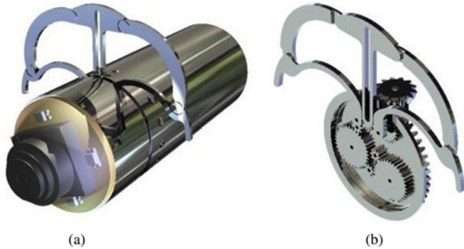
Fig. 3. (a) Holding mechanism concept which utilizes a vertically orientated micromotor to give the WCE the ability to overcome peristalsis and (b) 3-D internal view of the gear train.
